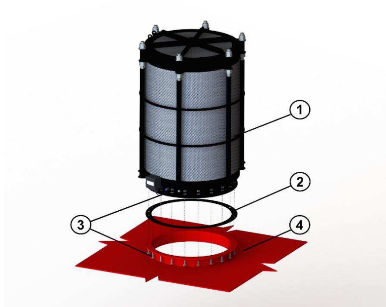
Fig. 13 - The Exploded View of the Round FLEX (1 - FLEX, 2 - flange gasket, 3 - fasteners, 4 - protected technology)
