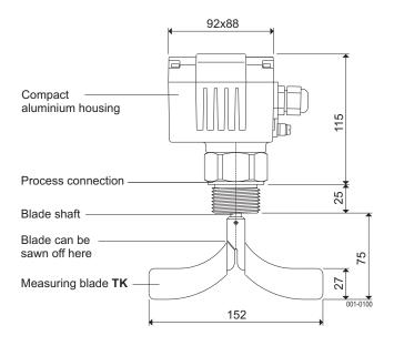
We recommend sawing off the plastic blade on one side, when using as empty indicator.
