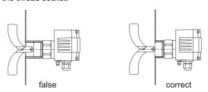
The level indicator has to be installed in this way that the jib won't be hit by the filling stream of incoming bulk goods.
