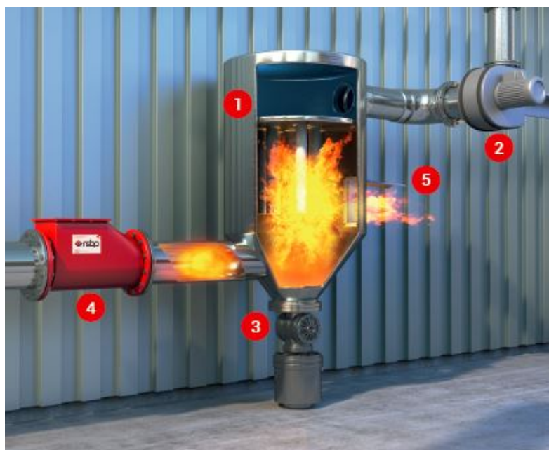
Figure 2 – Diagram of the working B-FLAP
